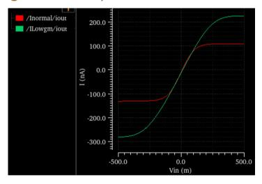
■ Try this in a 2<sup>nd</sup> transconductor. Compare in a dc simulation to your first version. Is the input range wider for same transconductance? (You must use different Ibias currents!)
