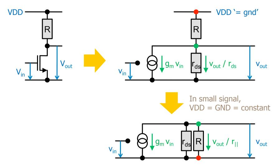
$\rightarrow$  R and  $r_{ds}$  act in parallel:  $v = -g_m \times (r_{ds} \parallel R)$
