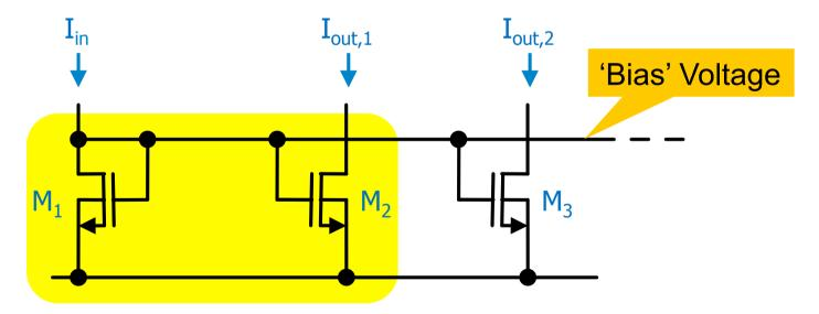
■ The gate voltage of the sources is called a 'Bias' Voltage
