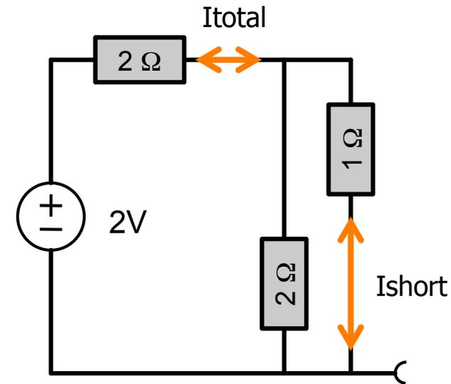
$$R_{total} = 2\Omega + 2/3\Omega = 8/3 \Omega$$
