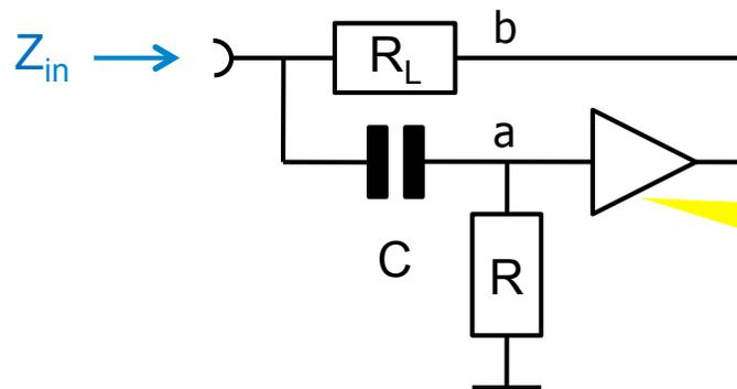
the triangle is a voltage amplifier with gain=1 ('follower'). It forces node b to the potential of node a
