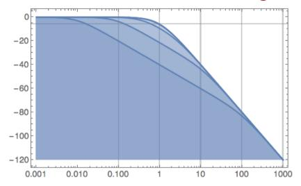
■ Plot the poles as a function of f where  $R_2 = R_1 f$ ,  $C_2 = C_1 / f$ , so that  $R_2C_2 = R_1C_1$ :
