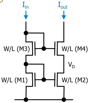
• What is the drain voltage V<sub>D</sub> of M2? Is that optimal?
