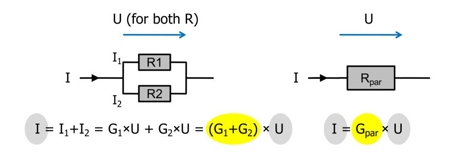
$$G_{par} = G_1 + G_2 \qquad \leftrightarrow \qquad 1/R_{par} = 1/R_1 + 1/R_2$$
