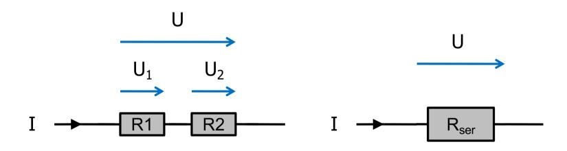
$$U = U_1 + U_2 = I \times R_1 + I \times R_2 = I \times (R_1 + R_2)$$
