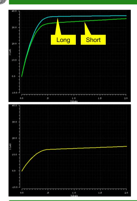
For the real MOS, the output resistance increases, when L is increased
