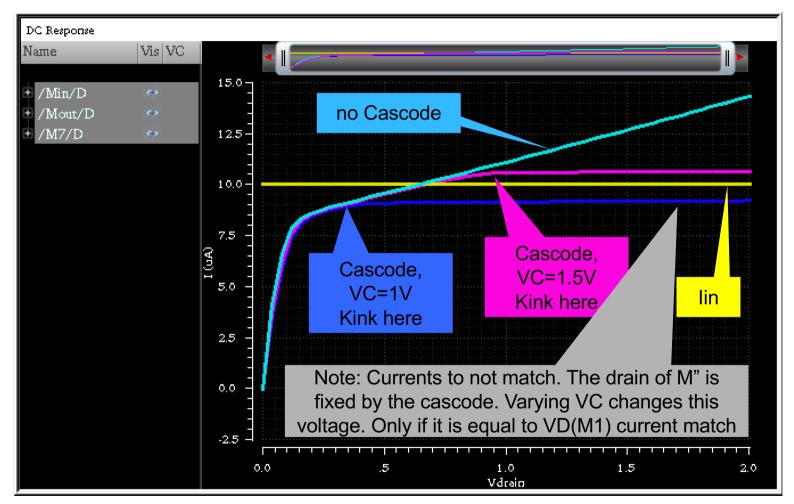
VC is 'ideal' if the onset of cascode action (the kink) is just above the saturation voltage of M2
