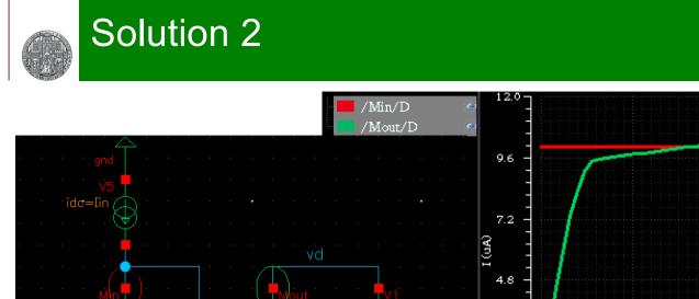
Currents are equal when Drain voltages are equal, i.e. when Vout = Vg (this depends on lin)
