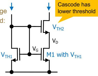
With a 'sufficiently low' V<sub>TH2</sub>, this works!
