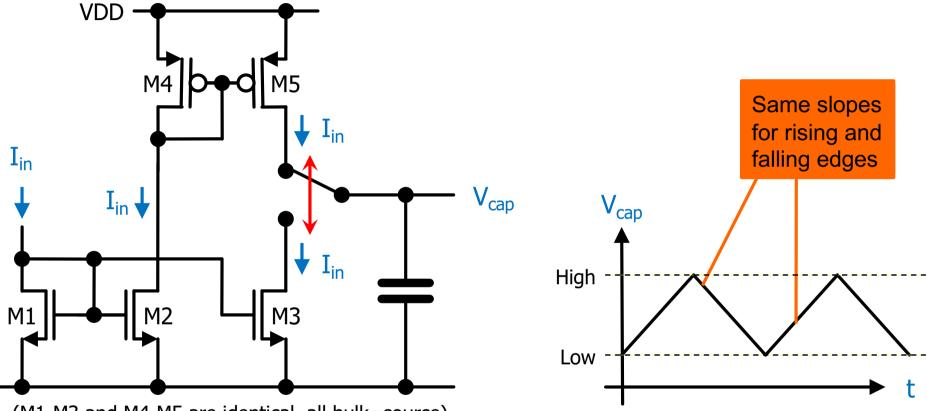
(M1-M3 and M4-M5 are identical, all bulk=source)
