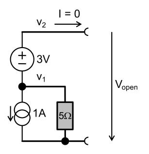
• Source:  $V_0 = V_{open} = -2 \text{ V}$ ,  $R_V = V_0 / I_{short} = 7 \Omega$
