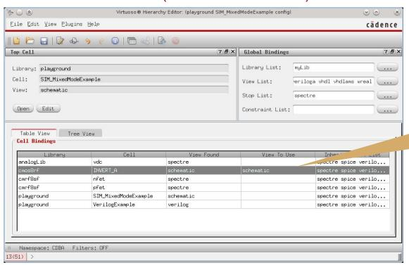
INVERT\_A has both a 'verilog' and 'schematic' view, the view to use can be specified here
