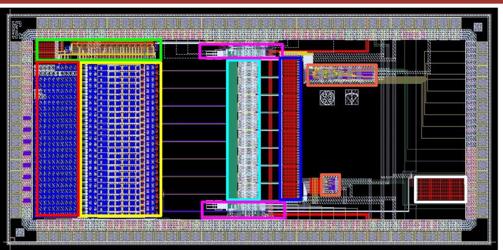
Bias circuitry (12 current DACs) 26 preamp/shaper channels Detector capacitors (5pF per block) 8 pipelined ADCs ADC control + bias 5.2 kBit shift register matrix Control + readout/decoder logic blocks Test circuits
