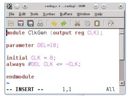
When the Verilog file is closed, Virtuoso offers to create a symbol if there is none (or modify it if it does not fit to the declared interface). Create the symbol.
