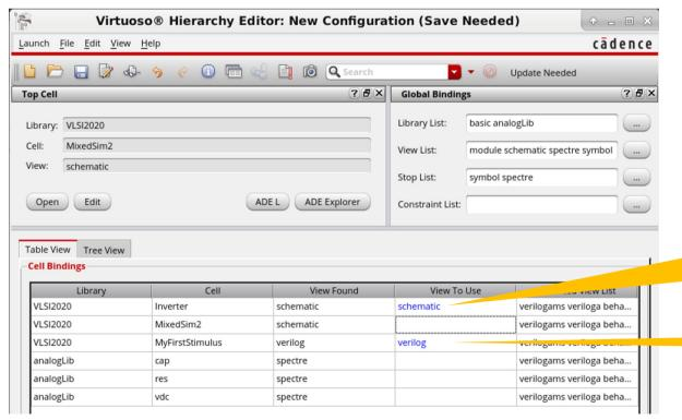
A cell can have several view, e.g. 'verilog', 'functional' or 'schematic'. The view to use is specified **here**
